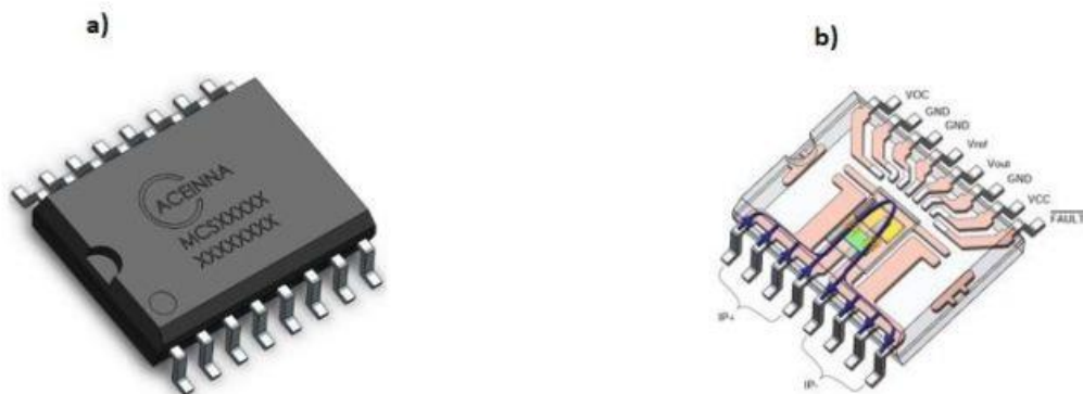
Figure 5: a) MCA1101 current sensor IC, b) Inside of MCA1101
