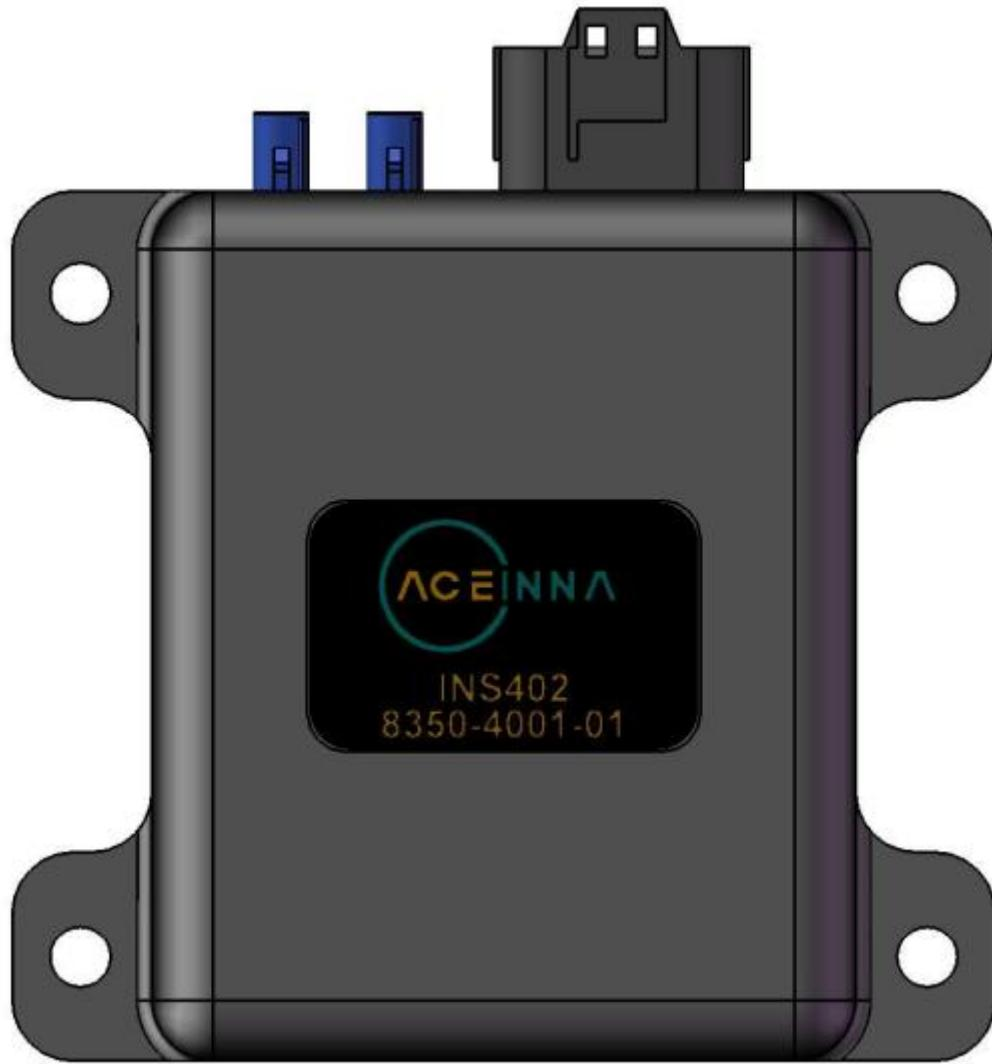
The Aceinna INS402 high-precision navigation system integrates a multi-constellation, multi-frequency Global Navigation Satellite System (GNSS) (supports GPS, GALILEO, GLONASS, Beidou, QZSS, NAVIC and SBAS), an Aceinna MEMS Inertial Measurement Unit (IMU) module IMU330ZA, and a single Cypress multi-core Cortex-M7 micro-controller (MCU) CYT4BFBCHD as the main processor. The INS402 system includes built-in proprietary GNSS RTK positioning engine and a proprietary INS navigation engine.
