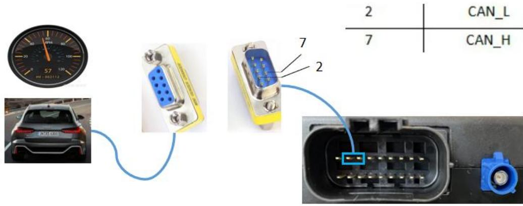
DB9 connector is recommended to connect with odometer signal line.
